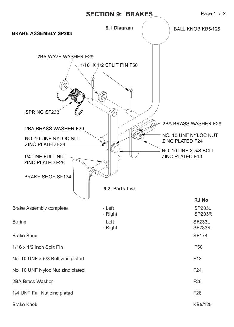
Check ball knob for security. Check levers for distortion. Check brazed joints for cracks. Check pivot shafts for distortion. Replace pivot bolts if necessary due to excessive wear. Ensure no oil/grease on brake pad.
